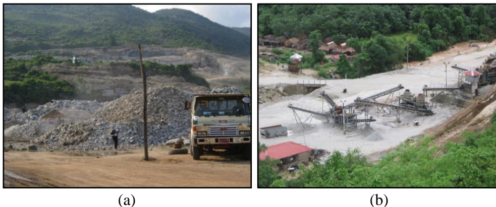
Figure 24: (a) Myanmar Ye Man Co. Ltd.,(b) Global Vertex Co. Ltd. extracting porphyritic biotite granite for construction and road materials and quality dimension slabs.
