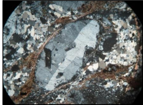
Figure 18: Orthoclase feldspar porphyroblasts surrounded by fine-grained recrystallized quartz and biotite flakes in gneissose granite, Between XN
